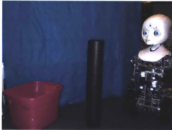
Figure 4-2: Example situation in which Nexi should deliver the upright cylinder on the floor to a bin.
