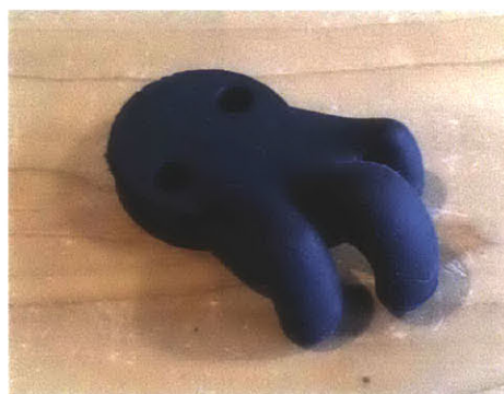
Figure 3-31: Foot prototype, urethane-iron hybrid material
