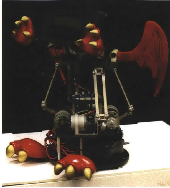
Figure 3-32: DragonBot V4 prototype with 3D printed aesthetics
