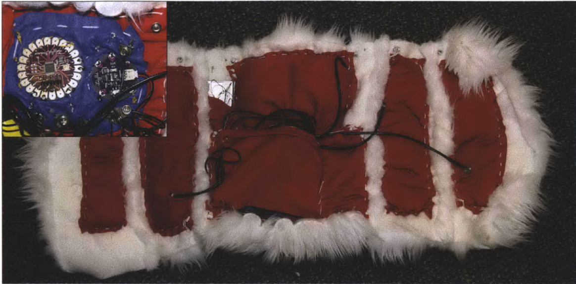
Figure 3-29: A prototype of a fur augmented with textile-based capacitive sensors
