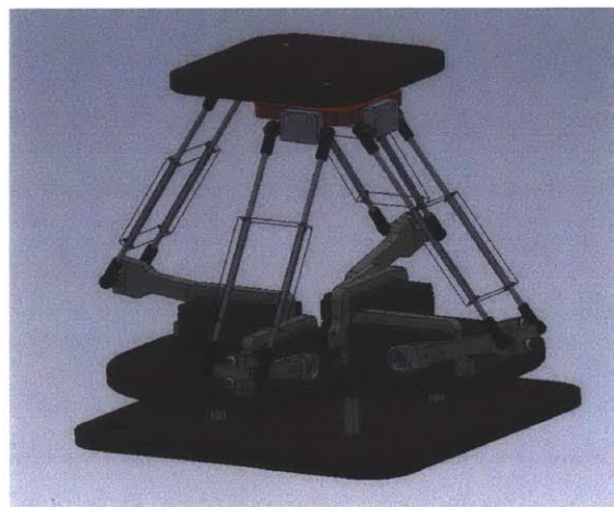
Figure 3-2: DragonBot solid-body model for initial prototype (V1)
