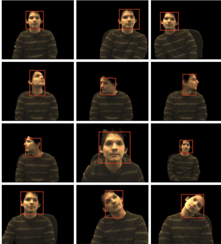
Figure 4-1: Output of the FaceTracker’s algorithm on a sequence of depth-color images. The red squares indicate the position and dimension of the faces.
