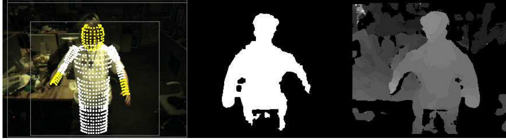
Figure 5-4: The robot currently has untethered real-time perception of both human upper arms and forearms, using the VTracker articulated body tracker.
