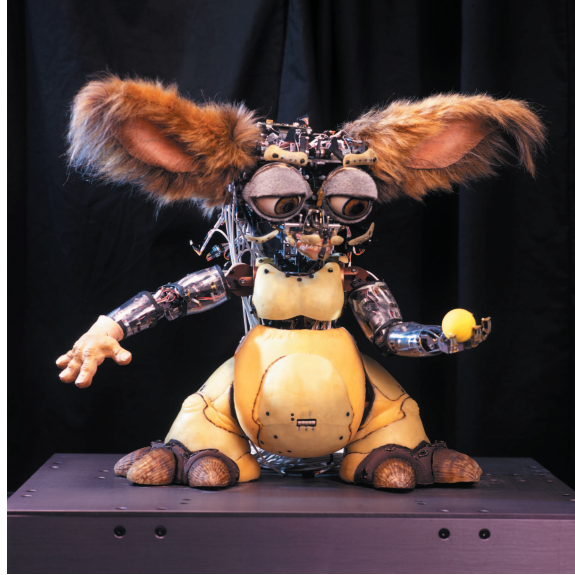
Figure 3-1: The Leonardo robot without its skin installed, showing some of its skeletal and outer shell structure.
