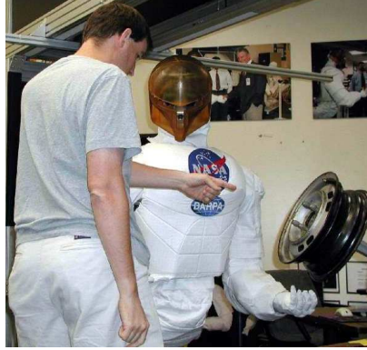
Figure 5-8: Execution of the pointing and labeling component of the Robonaut nut-tightening task. The four nuts are indicated by the human in order to label them with their sequence numbers, and the gestures then matched to the correct object referents simultaneously.
