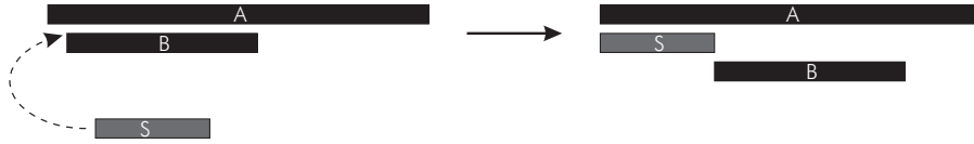
Figure 7-7: Insertion of a spacer interval S in order to precisely control the start point of B relative to A.
