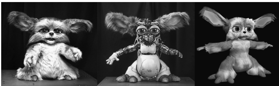
Figure 2. Leonardo, the robot and virtual simulator. Cosmetically finished (left), with mechanics exposed (center), and the animated model (right). Character design copyright Stan Winston Studio. Images copyright MIT Media Lab (left and right image) and Sam Ogden (center image).
